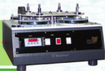
▣ Abrasion & Pilling Tester at DIU Textile Testing Lab
